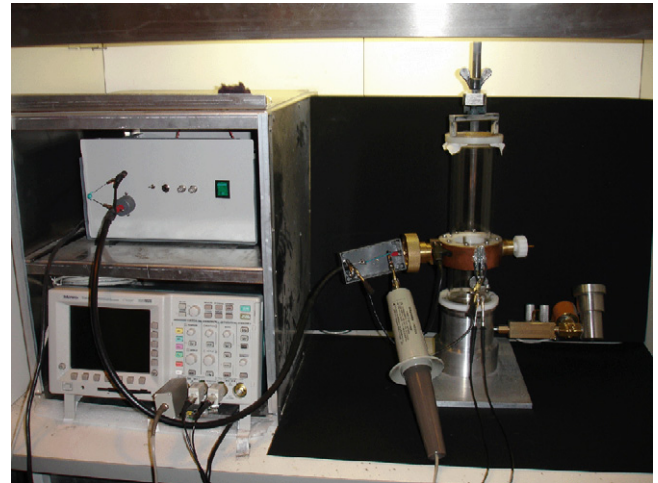
Fig. 3. The spark generator, the spark energy measurement system and dust explosion chamber. Further details about the set-up are given in Ref. [8].
